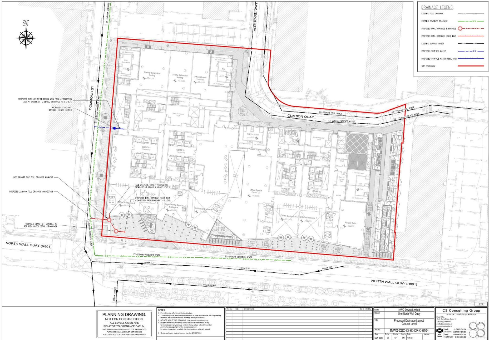
Figure 8. Proposed drainage layout – ground level
